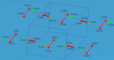
The infinite ionic chains in the crystal build by the (O – H...O)-fragments interacting by strong short H-bonds
